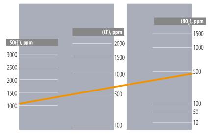
A model, shown in the second diagram, has been designed to predict the maximum concentration of chloride that can be permitted in water containing sulphate and nitrate ions before localised corrosion of 3CR12 takes place. A straight line, drawn between the concentrations of sulphate and nitrate, intersects the chloride axis at the maximum permissible chloride concentration for this water, at ambient temperature.
