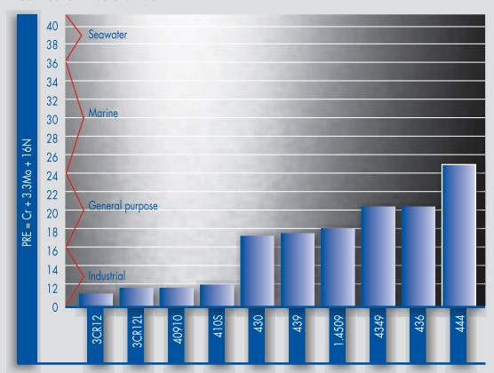
The above diagram summarises the corrosion resistance of the ferritic stainless steels produced at Columbus Stainless. For the standard ferritic stainless steels, the corrosion resistance is largely a function of the chromium content.
