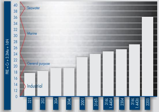
The above diagram summarises the corrosion (pitting) resistance of the austenitic and duplex stainless steels produced at Columbus. This would indicate that the corrosion resistance of the Cr-Ni-Mo austenitic types are all similar and suitable for marine environment applications.
